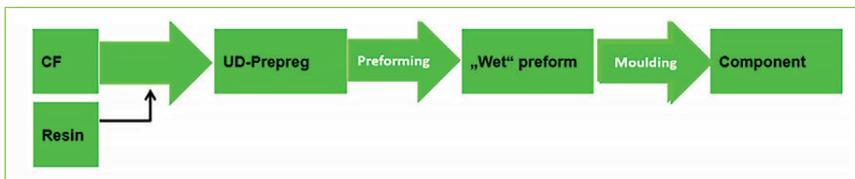
Fig. 2: Press Compression Moulding (PCM) sequence
