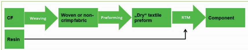
Fig. 3: Resin transfer moulding process (RTM)
