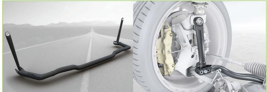
Fig. 1: CFRP stabilizers on the front and rear axle
